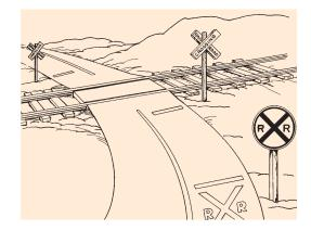
4. The DRIVER MUST STOP THE BUS BEFORE THE CROSSBUCK sign or signal at the crossing. On gravel roads there are no pavement markings or Stop Lines. The Stop Lines on each
